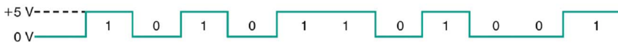
Digital signals (a) Telegraph (Morse code). (b) Continuous-wave (CW) code. (c) Serial binary code
